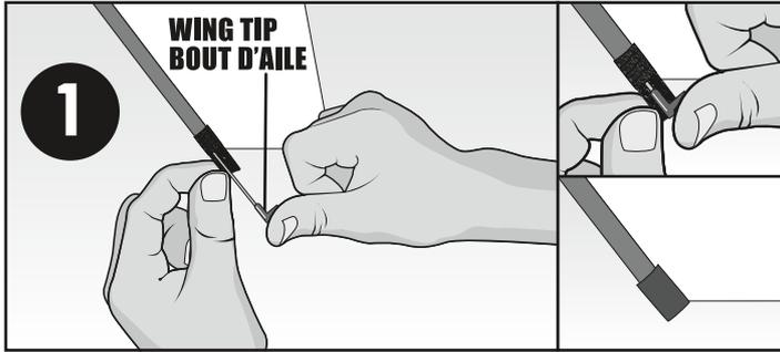
**1. Main Wing Assembly: Push in Wing Tip (Red) and fold over the Velcro Tab securely (left/right).
