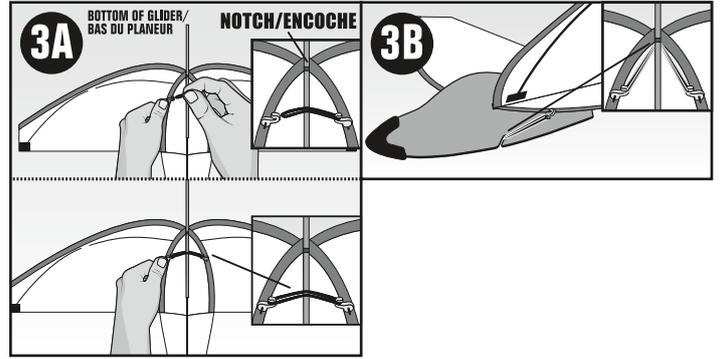
**3A. Lower Wing Assembly: Attach the Lower Wing Support Rubber Band to the opposite side of the Lower Wing.
