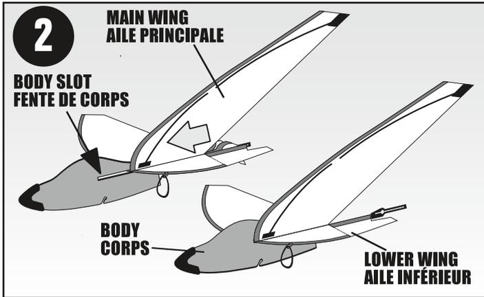
**2. Main and Lower Wings Assembly: Slide the Main and Lower Wings into the Body Slot
