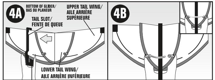
**4A. Tail Wing Assembly: Pass both Upper and Lower Tail Wings through Tail Slot.
