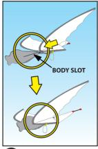
Main & Lower Wings Assembly: Slide the Main and Lower Wings into the Body Slot.
