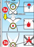
Tail Wing Assembly: Form an X with the Tail Wing. Slide under the Rear Center Peg (Red). The Smaller Bottom wings go under the Left and Right Rear Peg (Red).
